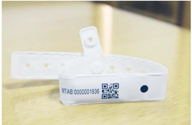
The tracking bracelet named iMSafe for remote monitoring and detection of people placed under the Quarantine Order in the country.
