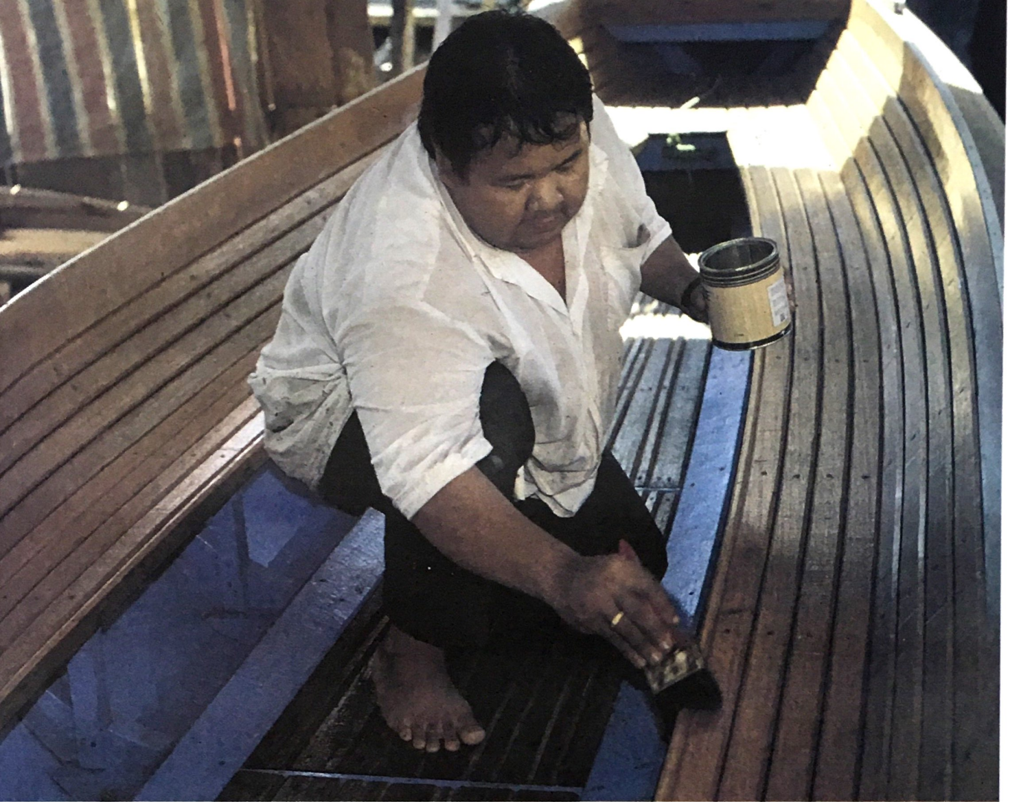
The inside of the boat – if it is designed to be a water taxi – is fitted with seats. The boatmaker is seen here coating the wood with varnish.
